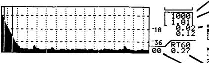
Display and/or print out a decay curve with RT<sub>60</sub> calculated from a section of curve you choose or...
