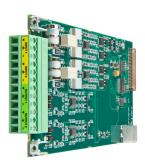
The DUAL-IO is a 4 channel modular analog IO card for use with Ivie MAP series devices. Each DUAL-IO provides 2 channels of balanced mic/line audio input, and 2 channels of balance line output, with software controllable gain, level, mute, phantom power, and signal inversion.
