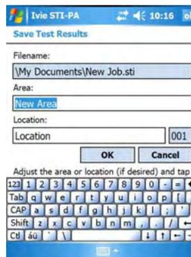
15. After sufficient tests are Averaged press the "Save" button to save the data to the Job file. Then press the "OK" button on the "Save Test Results."
