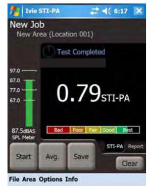
12. View the test results. If acceptable press the "Avg." button.
