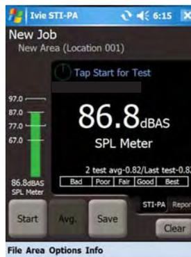
14. If acceptable, press the Avg. button for a total of two tests. Take additional test(s) and press "Avg" after each test.
