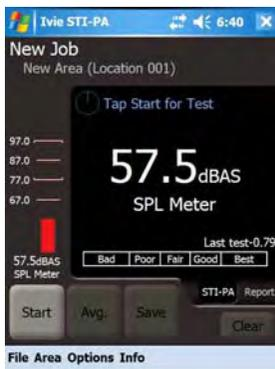
9. Check that the Ambient level is at least 20dB less than the Target playback level.
