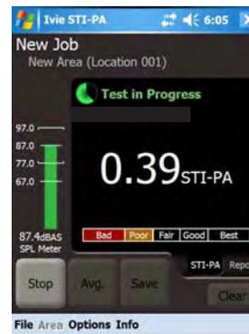
11. Monitor the test during the 15 seconds. No impulse noise should occur during the test.
