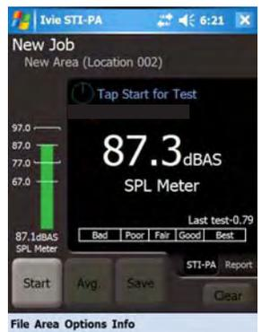
16. Start tests at a new location. Start, Avg, Start, Avg....., Save. Move to a new location. Start, Avg, Start, Avg....., Save.....
