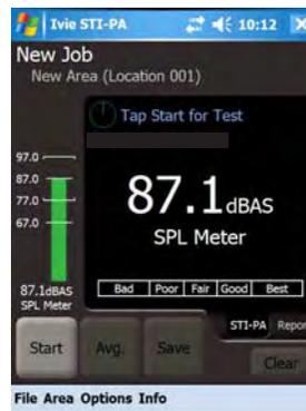
10. Adjust playback level of STI-PA in room for target of 87dB. Now press the "Start" button.
