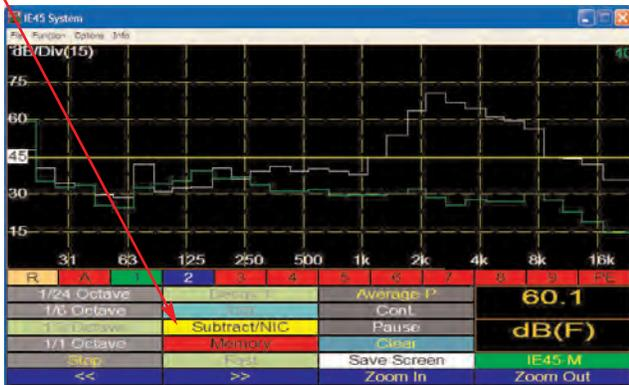
For NIC measurements, store the Source Room curve in Memory #1, and the Receive Room curve in Memory #2. Next, tap the yellow Subtract/NIC stylus button.
