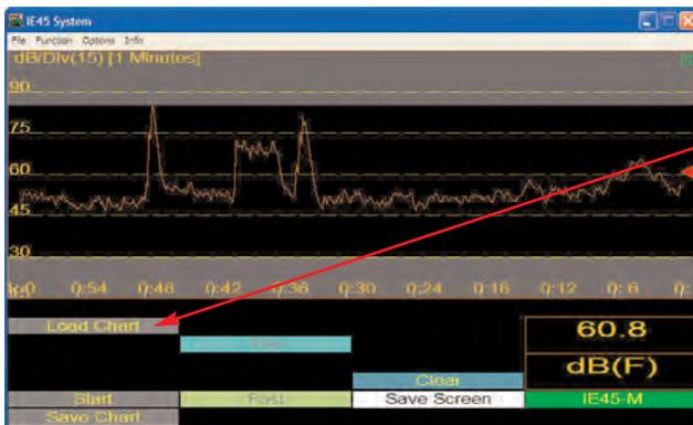
To view a saved chart, tap the "Load Chart" button. The screen to the right will pop-up allowing you to select the proper chart for viewing.
