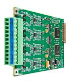
The QUAD-FIR is a modular analog output card with DSP processing for use with Ivie MAP series devices. Each QUAD-FIR provides 4 channels of balanced line level output with in-line DSP processing for programmable FIR filters. Audio channels are software programmable for filter coeficient files, and controllable for level, and signal invert.
