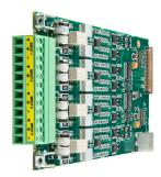
The QUAD-IN is a 4 channel modular analog input card for use with Ivie MAP series devices. Each Quad In provides 4 channels of balanced mic/line audio input with software controllable gain, level, mute, phantom power, and signal inversion.
