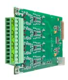
The QUAD-OUT is a 4 channel modular output card for use with Ivie MAP series devices. Each Quad-Out provides 4 channels of balanced line audio output with software controllable gain, level, mute, and signal inversion.
