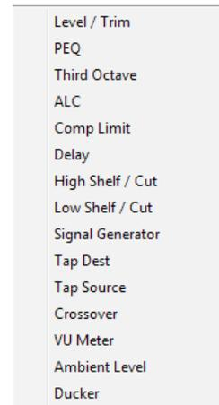
To add a processing element, left-click the plus icon to the left or right of the default level/trim icon, and select a processing element from the list. The new element will show up to the left or right of the level/trim icon depending on which plus icon was selected. To modify the location of a processing element, or to delete an element, right-click on the element and select 'Shift Right, Shift Left, or Delete'.
