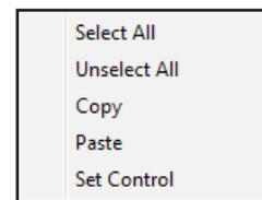
dramatically reduce the number of modes that may need to be defined. The 'Set Control' function helps to speed the definition of crosspoint conditionals by allowing all the crosspoint conditionals of a given output to accept a new control as the logic input of the conditional with a single command. The 'Set Control' command will allow the user to select a new control, and then paste that control as the control to be used for all of the crosspoint conditionals of that output.
