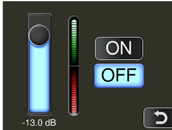
Notice the 'back' arrow in the lower right corner of the display. This will take the user back to the main page list display. Most display pages for complex, or named controls will use the entire page of the display, but some controls are simple enough to display from the main list page. For these controls, the Ivie logo and iTC-1 serial number will be replaced in the right half of the main page list, by the control.
