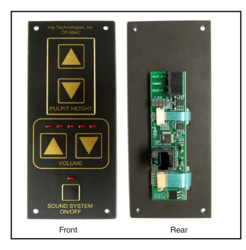
The CP-884C remote control is intended for use in Ivie LDS meetinghouse audio systems. The CP-884C provides the remote control functions for the Chapel portion of the system and replaces the CP-884. Connection to the CP-884C is by means of an RJ45 connector.
