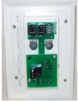
The **RMI-CC Wall Mounted 3-input Remote Control** is a wall mountable unit intended for installation in areas where control of up to three inputs (and an additional, local stereo to mono line input) may be useful.
